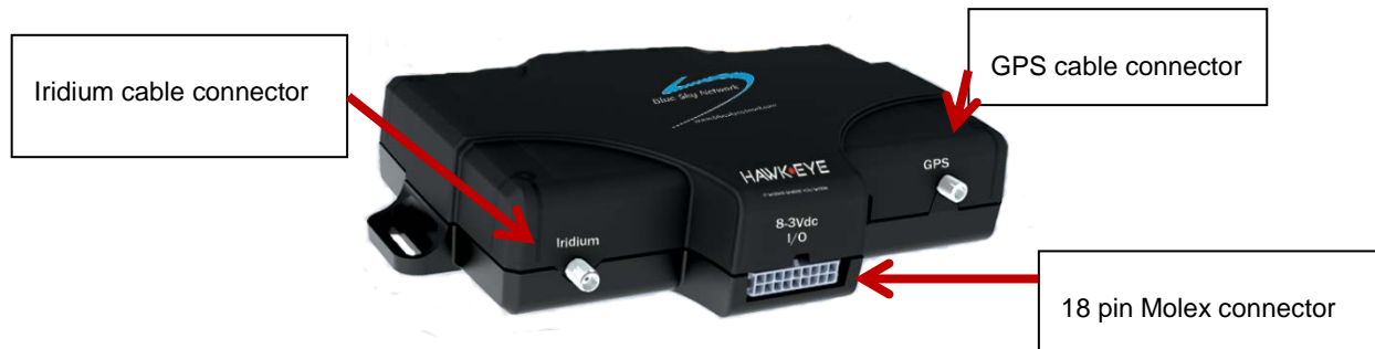
Figure 9: The HawkEye 5300 device has connectors for both Iridium and GPS cables.
