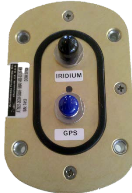
Figure 7: The back of the HawkEye 5300 antenna with dual inputs (capped) for GPS and Iridium.
