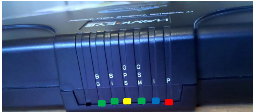
Figure 13: The HawkEye 5300's LED display.
